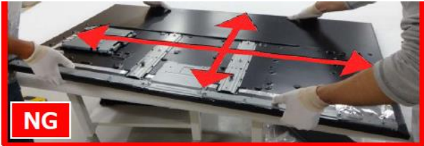
Moving at Horizontal Condition is NG
