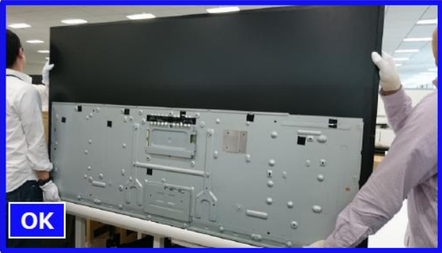
Move the Panel at Vertical Condition
