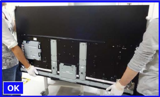
Move the Panel at Vertical Condition
