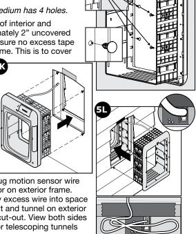
**5M.** Insert screw rods with hex nut completely through the four outer screw holes on exterior frame until hex nut is flush within screw hole.
