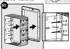
**5J.** Using a ¾6" drill bit, drill through side holes located inside exterior tunnel frame through exterior pet door frame. From inside of tunnel, push to insert a tunnel fastener into each hole you just drilled until head of fastener is flush with tunnel side.
