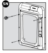
**50.** Insert finishing plugs into screw holes on interior and exterior frames. Align flat edge of plugs with outer edges of frame. Plugs will only fit one direction. Plug power adapter into connector on underside of interior frame. Route power adapter wire through wire guides in desired direction towards nearest power outlet.
