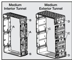
**3A.** For the Medium Passport™ Wall Entry Tunnel Kit, assemble two interior tunnel side panels (A) together by aligning arrows and snapping together. Repeat with remaining side panels. These are the sides of interior tunnel frame.
