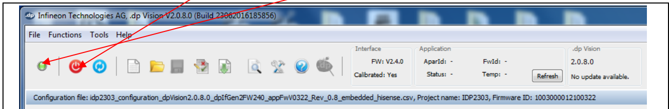
Figure 34 Power device On/Off button and device status
