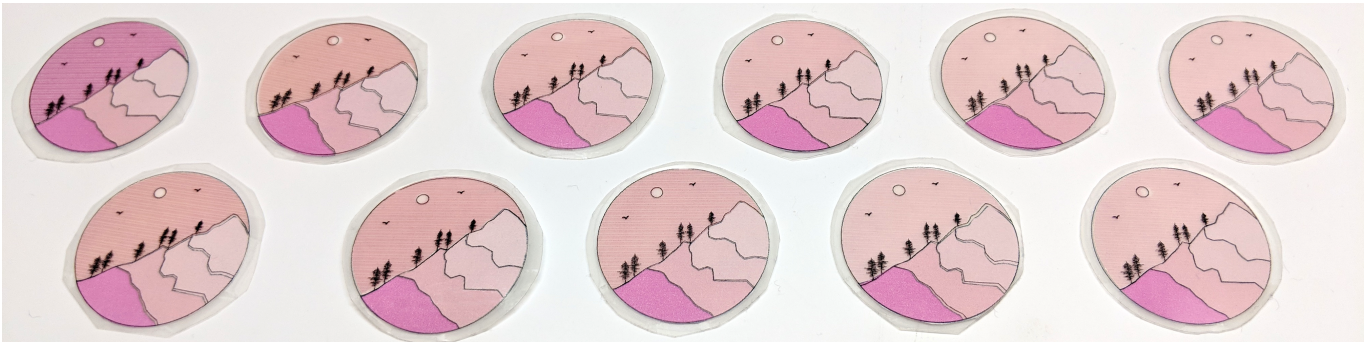
Figure 7. A photo of the actual EcoPatches used for the evaluation. The EcoPatches are sorted from left to right in increasing increments of 1.1 UVI-hrs. Note that the EcoPatches are covered with an additional clear layer to preserve their color for this photo.
