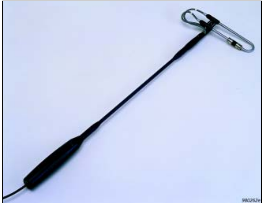
Fig.2 The sound intensity probe consists of: Dual Preamplifier Type 2683 and Sound Intensity Microphone Pair Type 4197. Here you can see it placed on an extension stem
