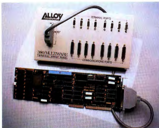
Alloy's IMP8 board supports eight users through the RS-232C panel.
