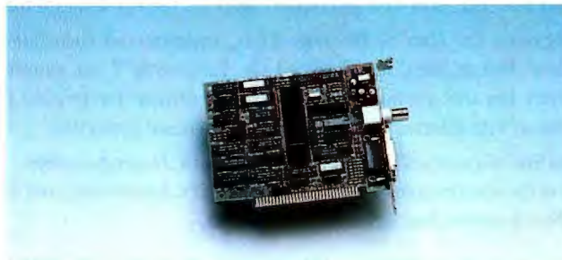
Photo 6: An EtherCard Plus from Western Digital ($399) allowed us to connect to either a standard Ethernet LAN coaxial cable or a Thin Ethernet cable.
