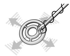
When pinpointing a target, try drawing an "X", as illustrated, over where the tone is induced.
