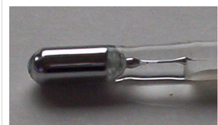
Close-up of a mercury-filled maximum thermometer. The break in the column of mercury is visible.
