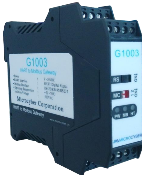
Figure 1 G1003 HART to Modbus Gateway Product Diagram
