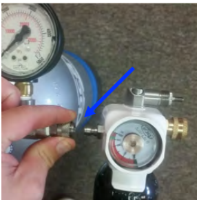
Figure 21: Pull back on the quick connect coupler to connect to and disconnect from the fill station.
