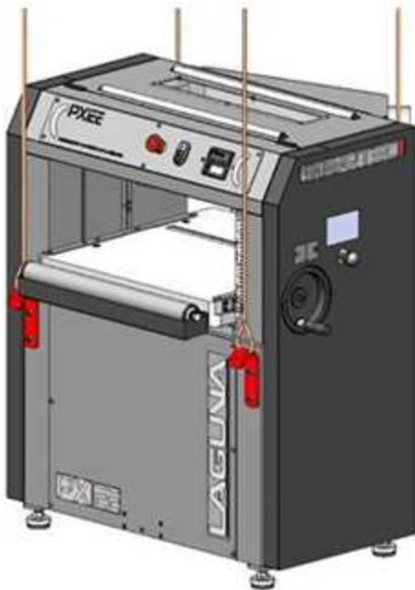
FIGURE 1: LIFTING PLANER WITH HOOKS AND HARNESS
