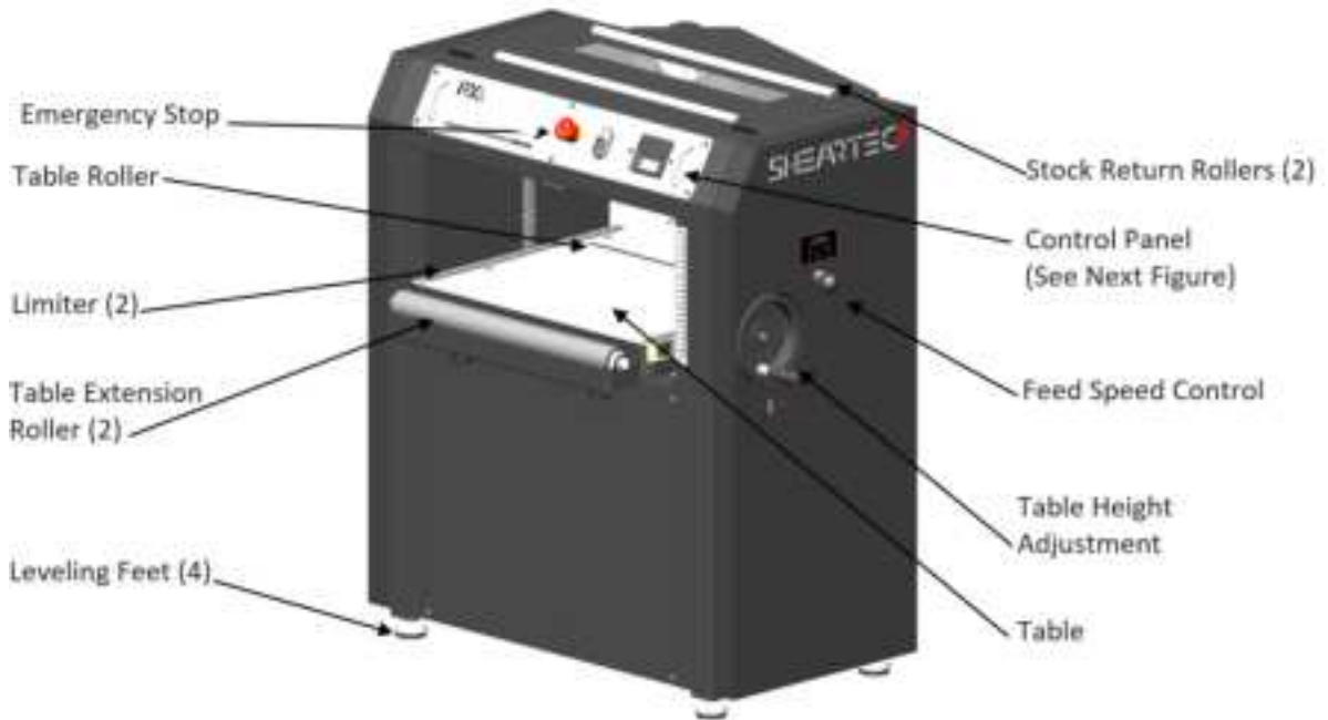
Figure 6: Main Components of PX20
