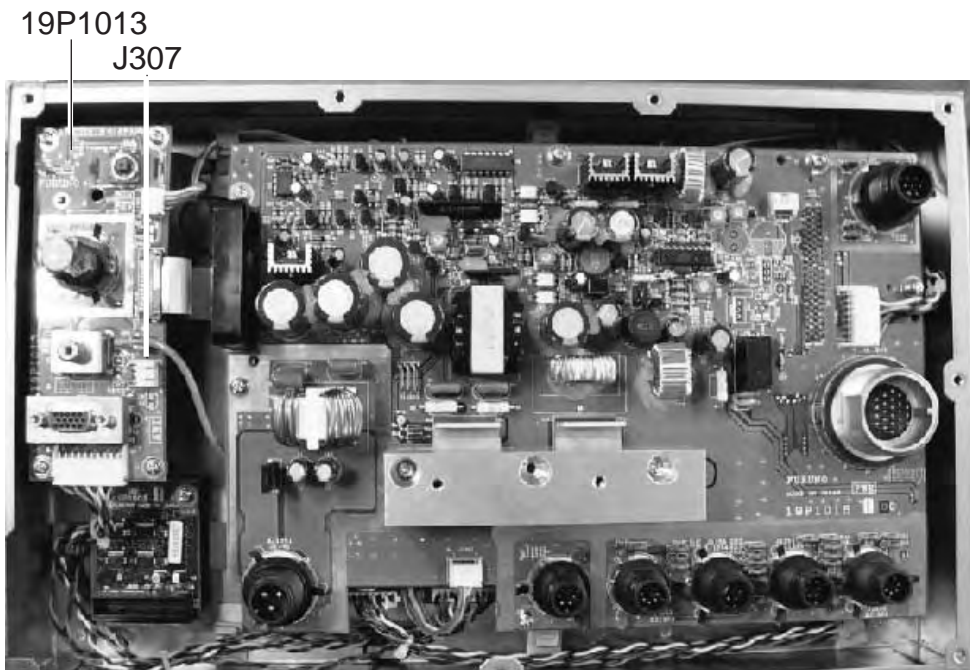
Processor unit (cover removed)
