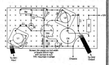
Fig. 2. The overlay built on 0.1in. perforated matrix board.
