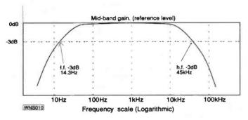
Fig. 4.7: A graphical representation of the gain bandwidth curve.
