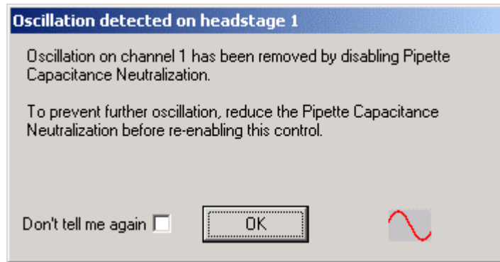
Figure 13. Oscillation detected message for I-Clamp mode.
