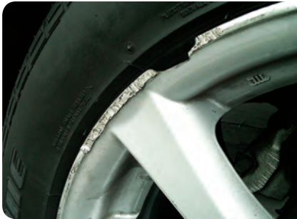
Damaged Alloy Wheel
