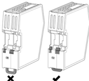
**Note:** Do not leave the module with the DIN-rail fastening mechanism in a fixed and open position. This may eventually wear the fastening mechanism out so it cannot be used efficiently. Be sure to push the DIN-rail fastening mechanism back into the fixed and closed position after demounting the module.
