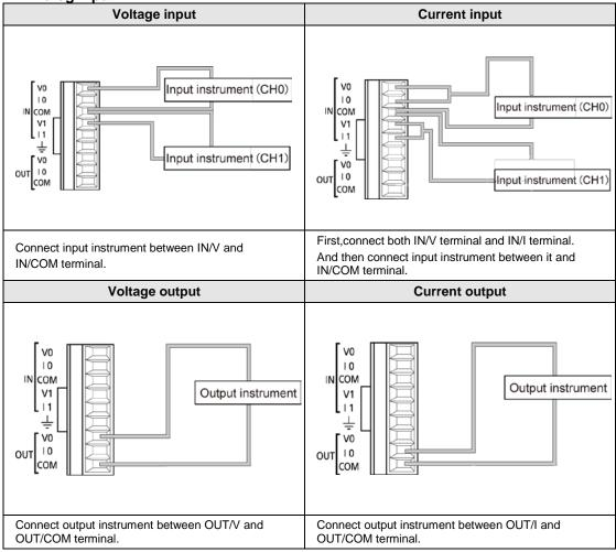
(Note 1):In the above figure, the input (CH0/CH1) and output CH0 are described as representative examples. The input (CH2/CH3) and output CH1 of A42 type also have the same terminal layouts.
