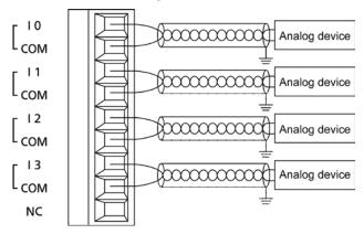
(Note):All COM terminals of the voltage output terminal block and current output terminal block are connected internally.
