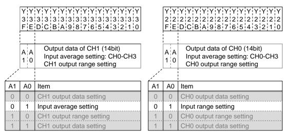
Set the contents allocated to CH0 to CH3 for the input averaging processing and input range by replacing the following 8-bit data with Hex data.
