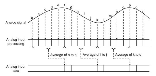
(Note):To make the explanation simple, the above figure shows the processing which averages data by five times. In the actual processing, calculation is carried out with the average of data for 64 times or 128 times.
