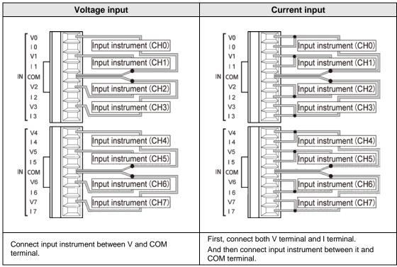
(Note 1): Two COM terminals are connected internally.
