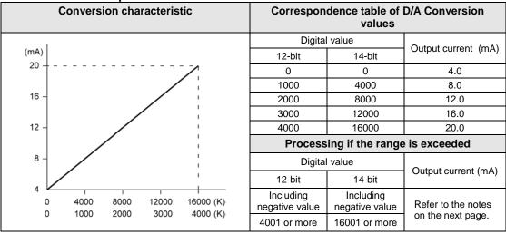
(Note):For the 12-bit mode, the values for FP0R-DA4 are shown. For FP0R-A21/A42 (12-bit mode), the range is 0 mA to 20 mA.
