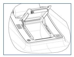
4. Take out the roll of used printer paper, and replace with new roll of printer paper. Make sure that the paper is placed and positions in the correct orientation, as shown below.
