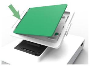
**Step 5 :**Press lightening connector cap into the tray and fasten locking screw if desired.
