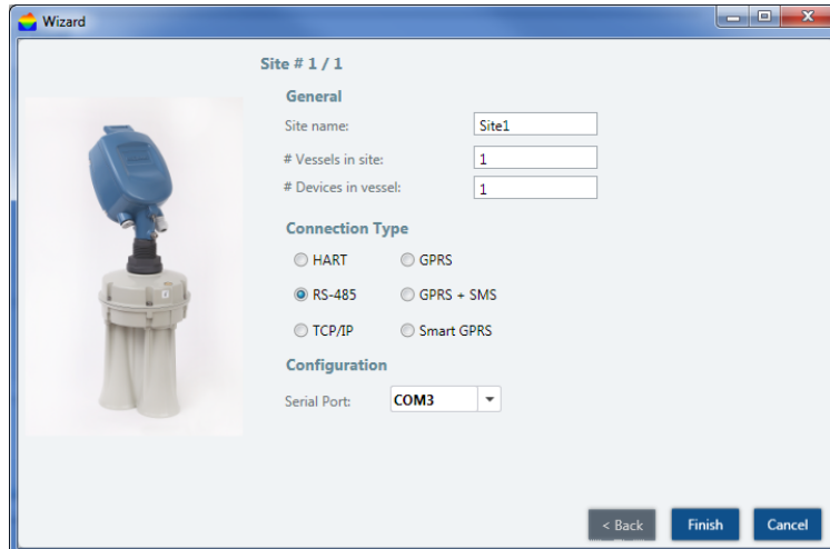
Figure 7-50. RS-485 Connection Type
