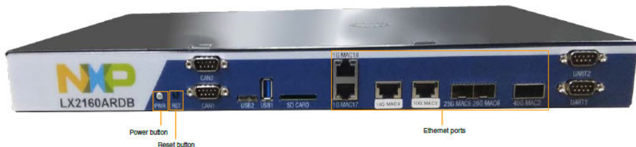
Figure 59. LX2160ARDB Ethernet ports
