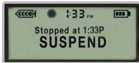
Pump in SUSPEND; notice the alarm icon
