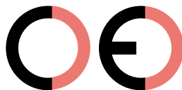
False CE Mark (too far)
