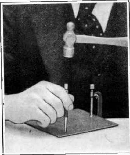
Fig. 3. Using the jig for laying out a panel
