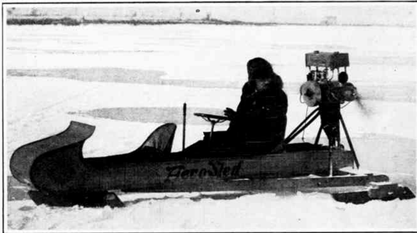
The Aero Sled depicted at the right uses a very compact power plant of double opposed form and a suitable aerial propeller, the entire outfit being suited for boat propulsion also
