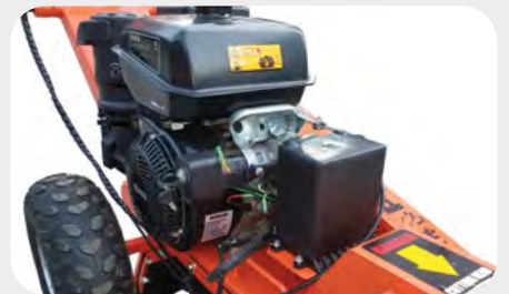
Dual direct V-Belt, high speed 3600 rpm drive.
