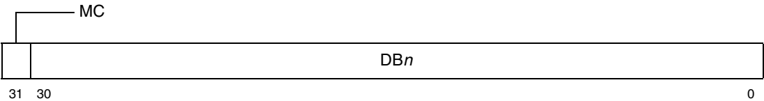
Figure 9-2. Inbound Doorbell Register (IDBR)
