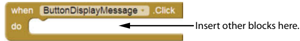
Figure 1-63 You Complete the Block by Snapping Other Blocks into the Empty Space. (Source: MIT App Inventor 2)
