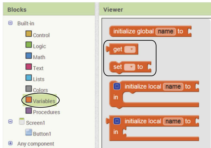
Figure 3-49 Blocks for Setting and Getting the Value of the Beverage Variable (Source: MIT App Inventor 2)
