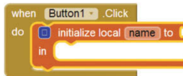
Figure 3-45 Insert the initialize local name to Block Inside the Desired Event Handler (Source: MIT App Inventor 2)
