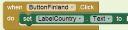
Figure 2-35 The set LabelCountry.Text to Block Snapped Inside the Click Event Handler (Source: MIT App Inventor 2)
