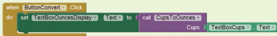
Figure 6-51 The Completed Click Event Handler for the ButtonConvert Component (Source: MIT App Inventor 2)
