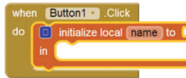
Figure 3-41 Insert the initialize local name to Block Inside the Desired Event Handler (Source: MIT App Inventor 2)
