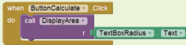
Figure 6-37 The Completed Click Event Handler for the ButtonCalculate Component (Source: MIT App Inventor 2)
