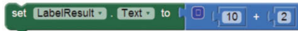
Figure 3-10 Displaying the Result of the + Operator in a Label (Source: MIT App Inventor 2)
