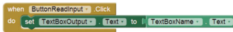
Figure 3-6 The Modified Click Event Handler for the ButtonReadInput Component (Source: MIT App Inventor 2)
