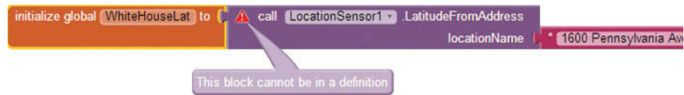
Figure 12-10 Do Not Use in a Variable's Initialization Block (Source: MIT App Inventor 2)
