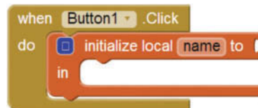
Figure 3-36 An initialize local name to Block Placed Inside a Button's Click Event Handler (Source: MIT App Inventor 2)
