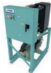
YCSE Water to water heat pump Screw compressor / R134a Hot water up to 55°C Heating capacity: 170 to 300 kW
