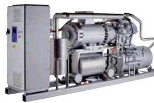
HeatPAC recip Variable-Speed Drive Reciprocating compr. / R717 Hot water up to 70°C Heating capacity up to 1200 kW at 40°C source
