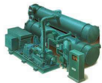
CYK HP / Titan OM HP Water to water heat pump Centrifugal compressor / R134a CYK HP: Hot water up to 70°C Heating capacity from 2500 to 7000 kW Titan OM HP: Hot water up to 90°C Heating capacity from 5000 to 20000 kW
