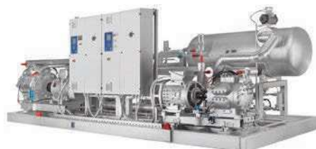
HeatPAC Custom Two-stage cascade VSD Screw compressor / R717 Hot water up to 90°C Reciprocating compressor / R717 Hot water up to 70°C Heating cap. up to +3000 kW at 40°C source
