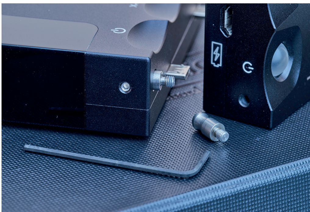
Two connectors are screwed into the HUGO, then the 2go is plugged in and secured with two allen screws
