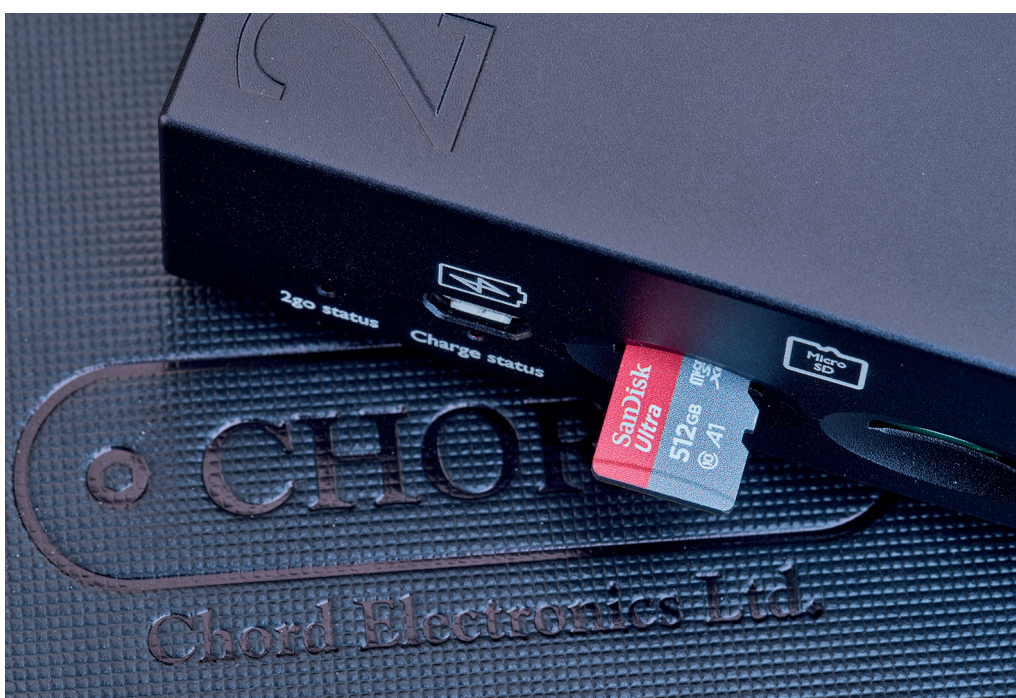
Next to the two slots for the micro SD cards is the micro USB charging socket of the 2go
