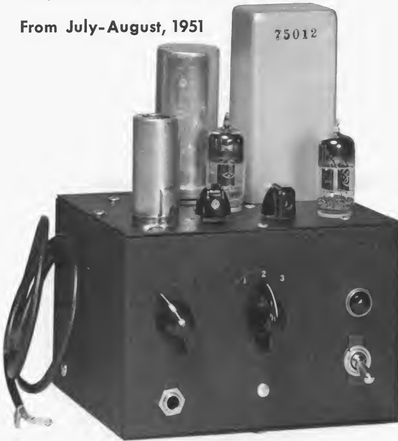
Fig. 1. Front view of the Signal Slicer. The input cable is at the left of the unit.
