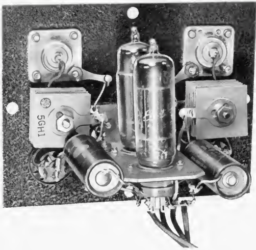
Fig. 4—Components of Dioplex mounted in space-saving arrangement
