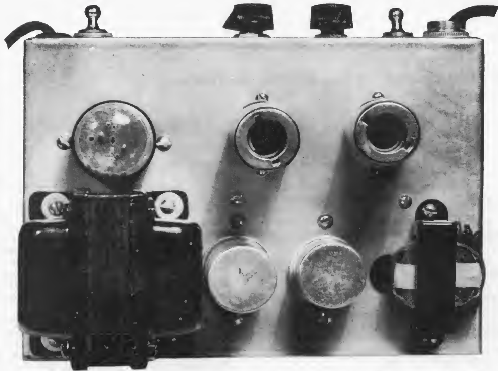
Fig. 5. Top view of the Logarithmic Compressor. The audio section is on the right and the power supply section is on the left.
