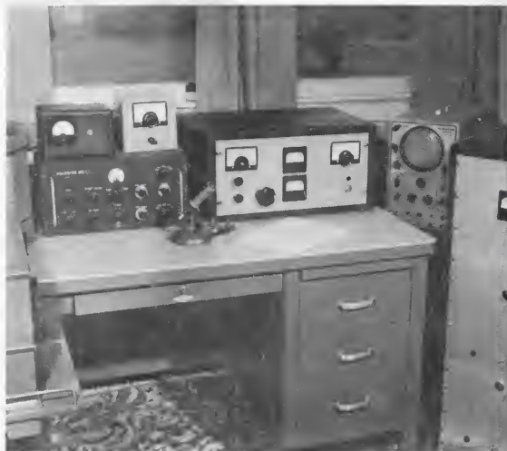
COMPLETE STATION at K2IOW with the Compact Triode Kilowatt at the right side of the operating desk. Other equipment includes an NC-240D receiver and speaker (extreme left); the 6L6-GC exciter which drives the 810 final; indicator for SWR bridge and High-C Bandswitching VFO atop the exciter; 5-inch 'scope for monitoring; and a 3-foot-high rack cabinet containing (top to bottom) class B GL-805 plate modulator, high voltage supply for the modulator, and a 2,000-volt DC supply for the 810 final.
