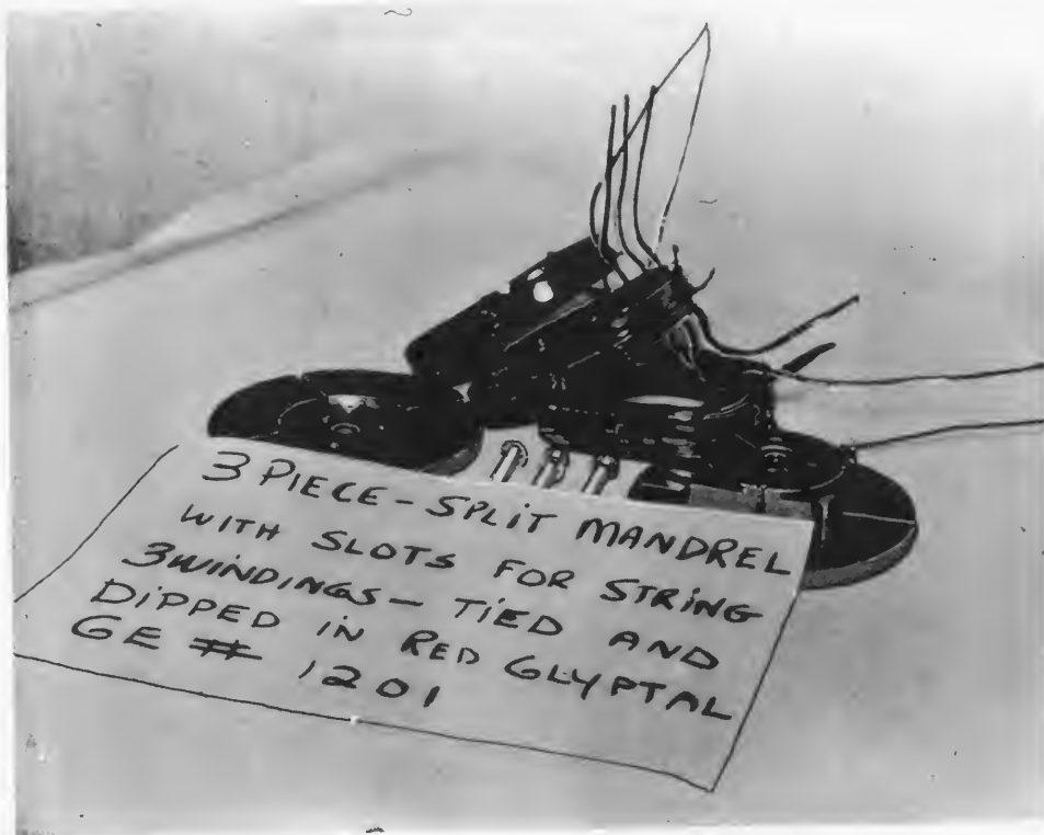
FIGURE NO. 2. VIEW OF WINDING MANDREL AND ONE SET OF COMPLETED COILS.
