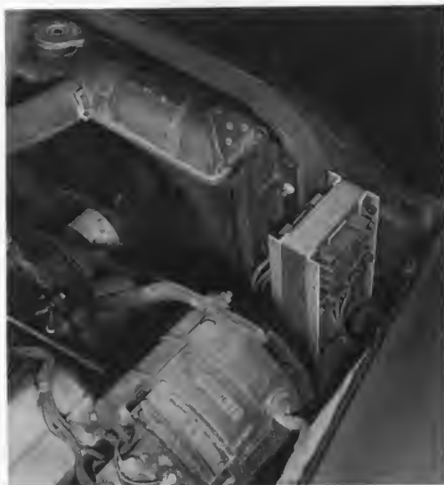
ENGINE COMPARTMENT VIEW of W8DLD's station wagon, showing Leece-Neville alternator in foreground and 3-phase distribution transformer mounted just ahead of it next to radiator.
