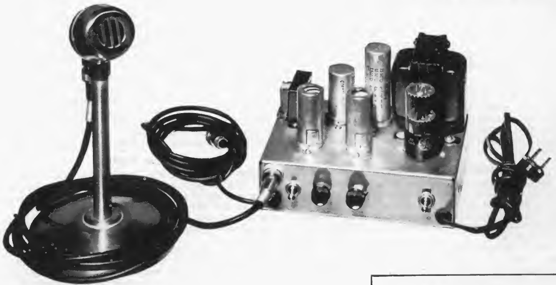
Fig. 1. The Logarithmic Compressor ready to plug into your present microphone jack. Controls are, left to right, in-out switch, compression control, output control and a-c on-off switch.
