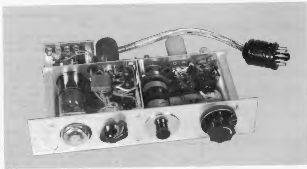
FIG. 1. SIDE VIEW of the COMBO MONITOR unit. Corner posts connecting the panel and chassis are 3 inches long. Those for the 2 x 2¼-inch mounting plate for the 1-megohm potentiometer are 1½ inches long. All posts are tapped for 6-32 screws at both ends.
