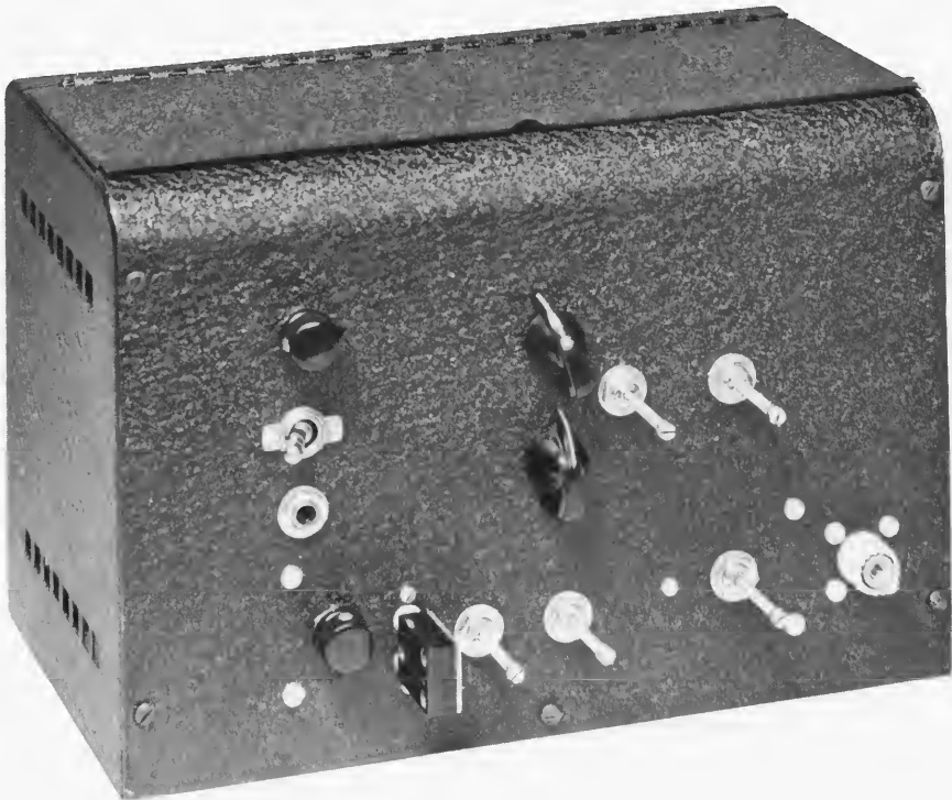
Fig. 1. Front panel view of the SSB Jr. For single-frequency operation none of the controls need be adjusted (except the audio gain control). Front-panel mounting of the controls permits a compact physical layout to be obtained.
