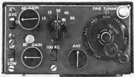
PANEL VIEW PHOTO of the bondswitching converter. Only the controls marked "RF GAIN," "ANT.," and "80-40-20-15-10" (the bandswitch) actually control circuits in the converter.
