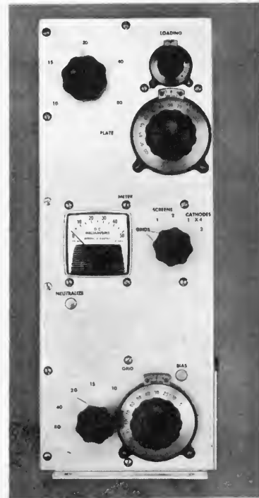
PANEL VIEW of the linear amplifier. Note that grid and plate bandswitches have separate knobs, and are not ganged. Snap-in buttons cover the holes through which the neutralizing capacitor ( C_2 ) and bias potentiometer are adjusted.
