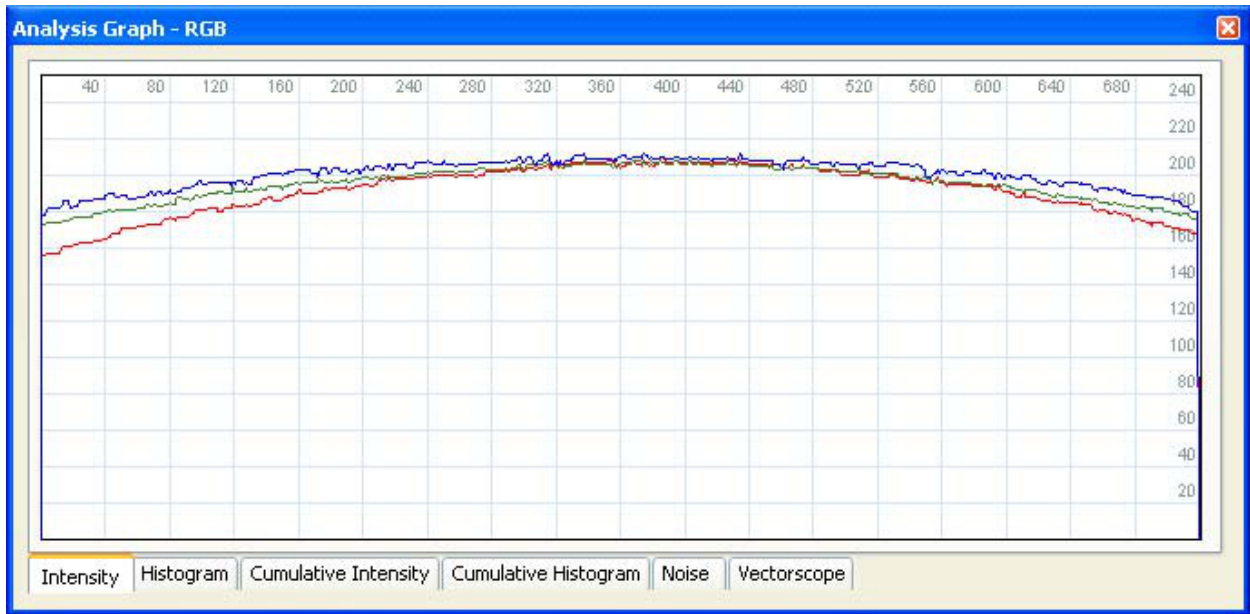
Figure 30. Intensity Graph after Increasing Integration Time
