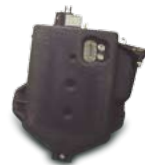
CFM56 engine reservoir
