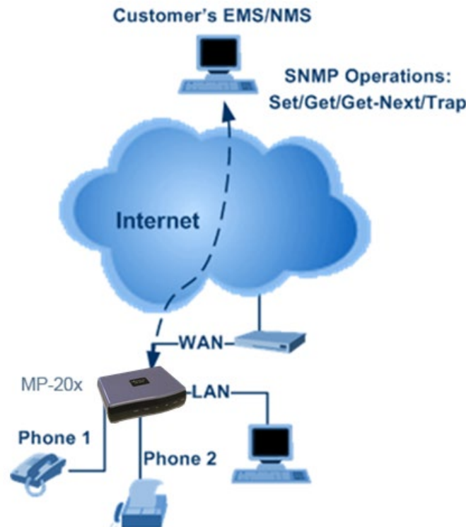
Figure 14-13: SNMP Network Architecture
