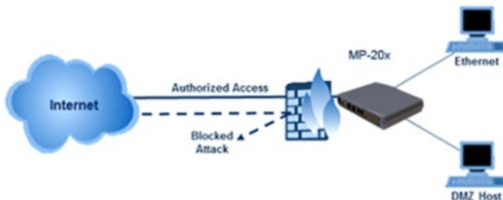
Figure 15-1: Firewall in Action
