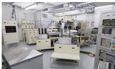
Dry etching facilities. The equipment visible at left controls the F 2 gas, while the equipment in the center supplies the gas
