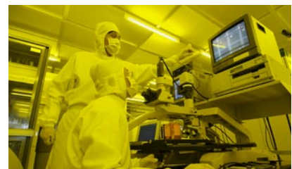
Using a microscope to inspect the surface quality of the TFT LC panels after the dry etching process with F 2 gas
