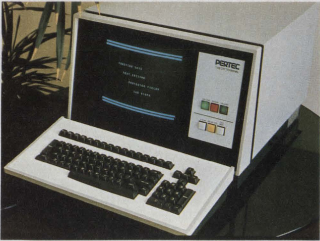
A microprocessor-controlled terminal with flexible data-communications protocol is the Pertec 7100.
