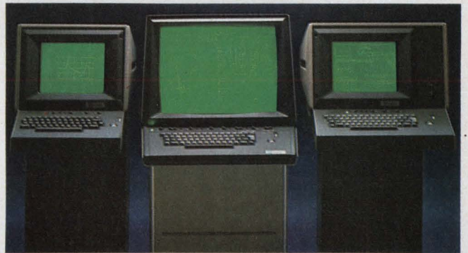
Tektronix makes a large selection of low-cost graphics terminals. Left to right are the 4010-1, 4014 and 4012. The 4014 has a 19-in. screen.
