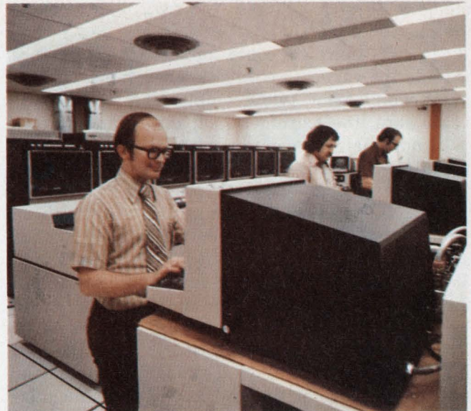
Programming tasks are made easier in this CDC Star-100 through the use of virtual memory and a very high-level instruction set. APL language is used.
