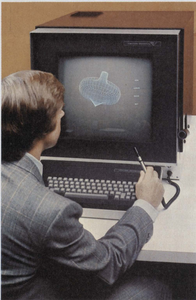
The Series-3 display terminal from Vector General provides hardware modularity and three-dimensional graphics. This terminal can also be obtained with a different CRT that provides a color display.
