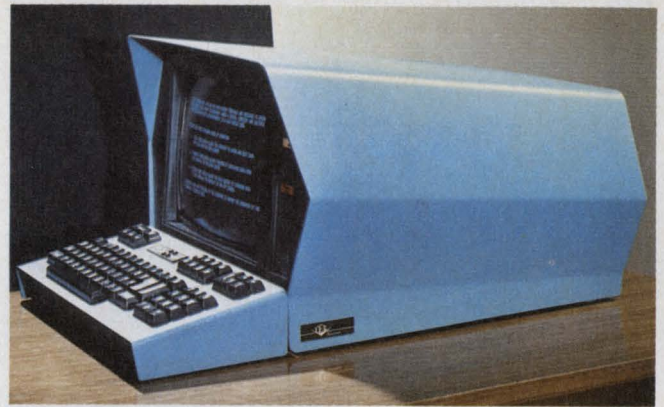
The Model 455 from TEC, Inc., is a smart terminal with a large character set and a full range of editing functions and cursor controls.
