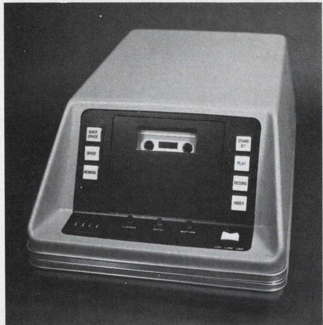
ICP's 3321 Termicette is a cassette peripheral that offers data rates of 110, 150 and 300 baud and has a gap-stop feature that provides automatic stop in a file separation gap without the use of special codes.
