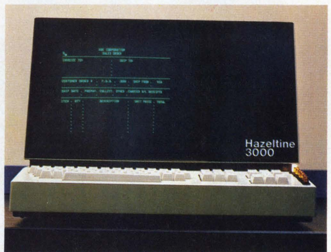
Hazeltine's 3000 is a smart terminal with a programmable communications interface. The interface provides the polling discipline compatible with the communication network.
