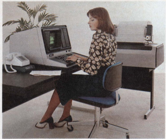
Sycor's 350 intelligent terminal contains a pair of built-in floppy-disc drives and a range of interfaces for other peripherals.
