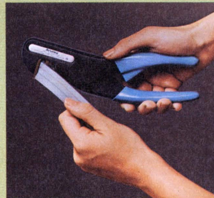
Pre-set compression cycle assures connection reliability.
