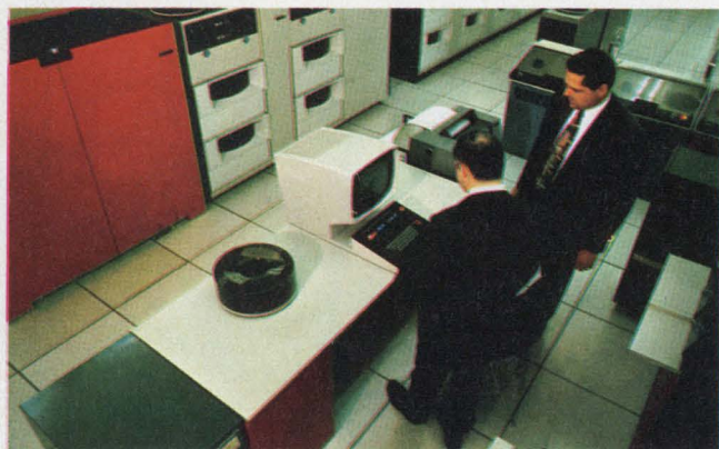
Distributed processing is found in the architecture of this IBM 370/125. Functions are assigned to I/O, arithmetic, and diagnostic processors.
