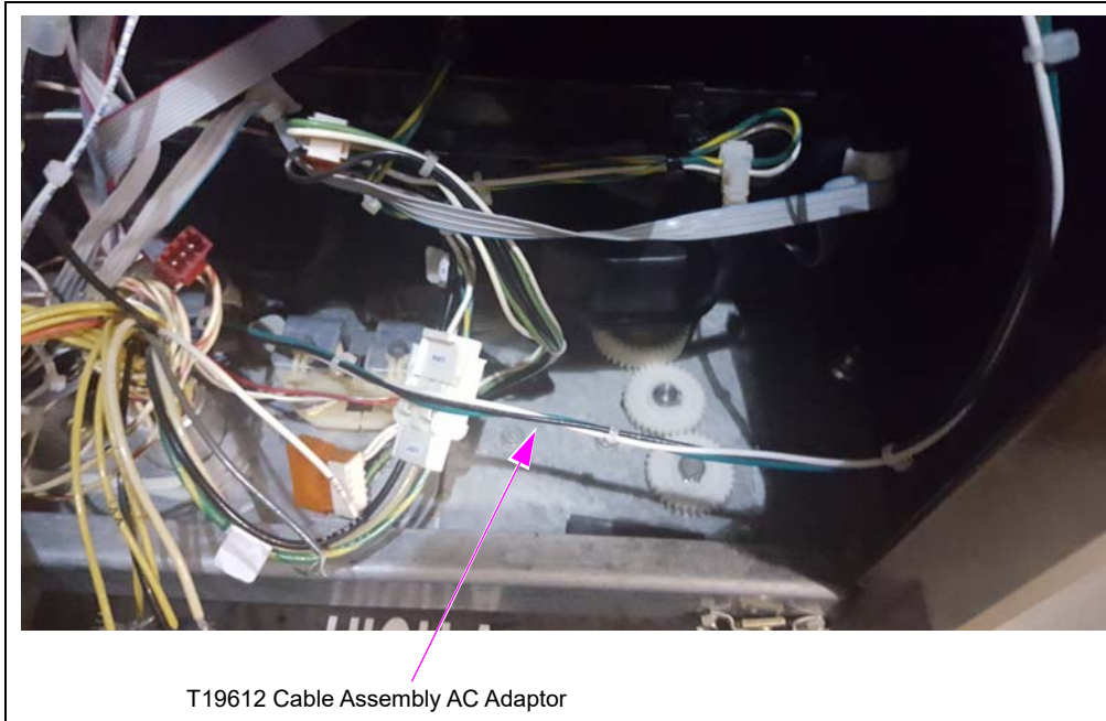
Figure 13: AC Power Distribution Cable Connection
