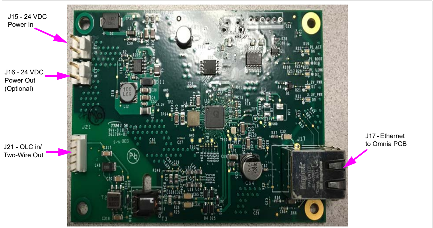
Figure 4: DCM3 Connections
