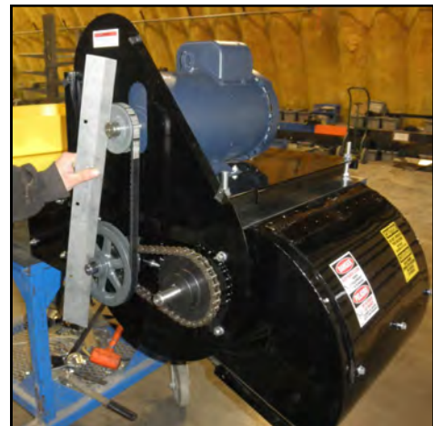
Lay a straightedge across pulley faces
