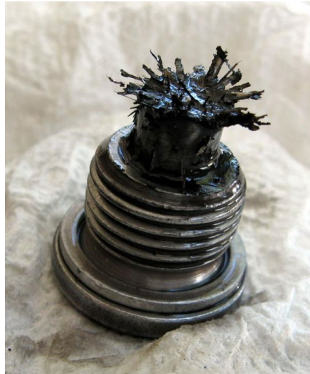
Figure 2: Abnormal levels and size of particulate warrants further investigation of gearbox components
