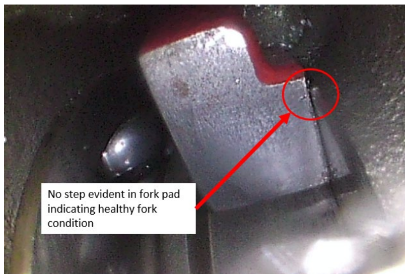
Figure 9: Acceptable Shift Fork
