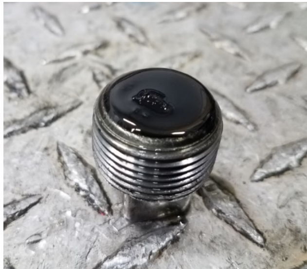
Figure 1: Normal sludge and particulate on magnetic drain plug
