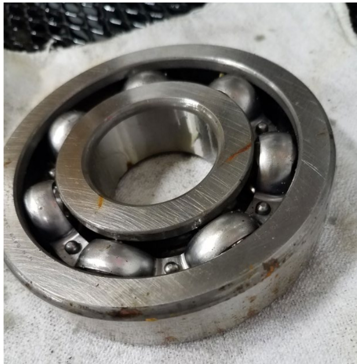
Figure 5: Bearing with signs of rust and corrosion indicating a replacement bearing may be needed.
