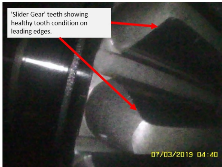
Figure 7: Acceptable slider gear teeth
