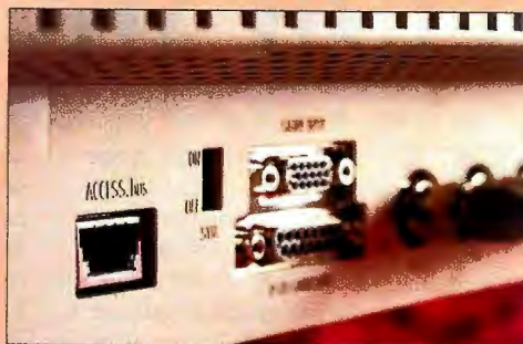
NEC's Multisync XE21 features an Access.bus connection (shown above) for hassle-free installation.
