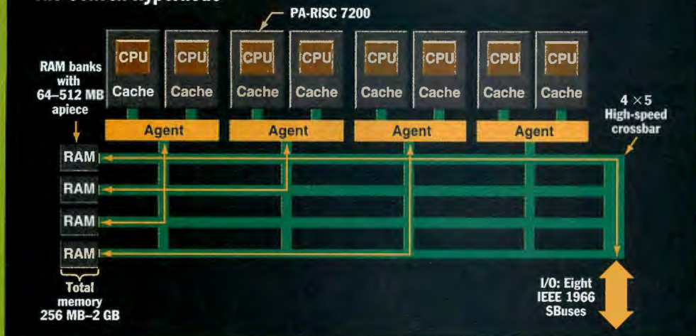
Top: A crossbar minimizes bus contention for RAM.
