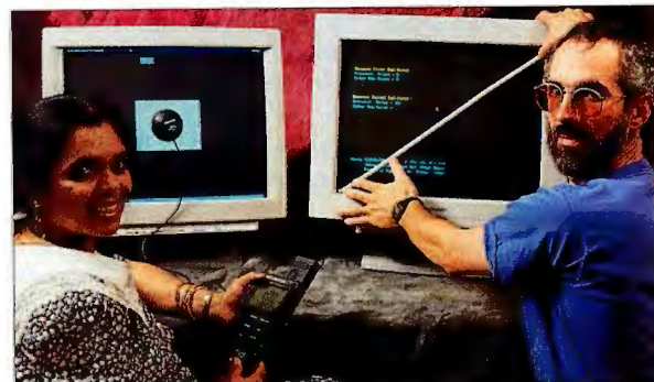
NSTL's Chandrika Mysore (left) measures the contrast ratio using a Tektronix Lumacolor II J18 Photometer, and Tom McAndrew measures the active display to calculate the distortion.
