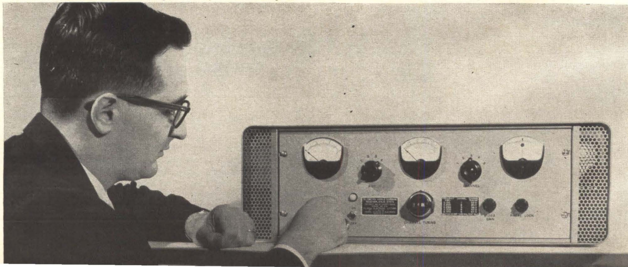
SSB TELEMETRY receiver using afc loop is tuned by author
