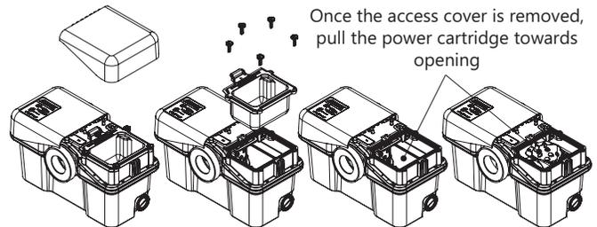
Once the access cover is removed, the power cartridge can be slid toward the opening by grasping the handle of the basket and pulling to the right toward the opening. In some instances, debris might be caught between the tank and the basket so some manipulation might be required.
