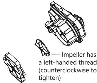
**Note:** the impeller has a left-handed thread. To remove, use a slotted screwdriver to hold the shaft and turn the impeller clockwise.
