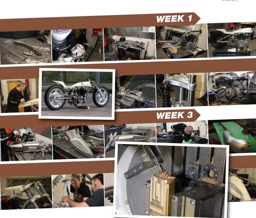
clean without the slightest dent in it. Our forming block was the milled plastic tank. Hours were spent in careful hammering and welding."
