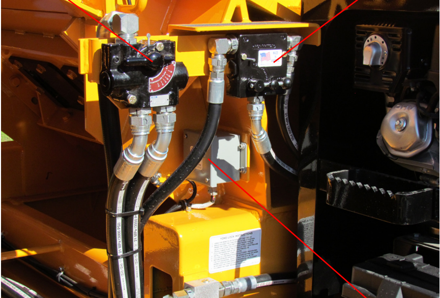
Feedwheel Flow Control Valves
