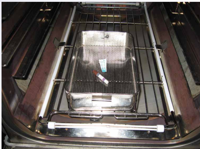
Figure 1. Biological indicator process challenge device for routine testing of immediate-use steam sterilization cycles in 270°F/132°C vacuum-assisted steam sterilizers using an open, perforated mesh bottom instrument tray
