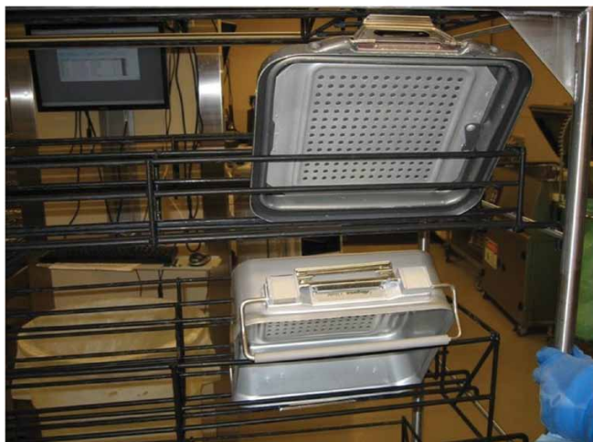
Figure 5. Rigid sterilization containers incorrectly loaded into washer-disinfector
