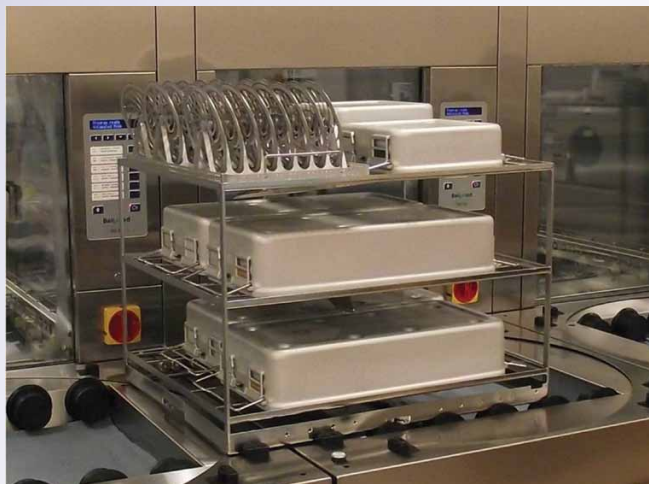
Figure 6. Correct disassembly and loading of rigid sterilization container in washer-disinfector
