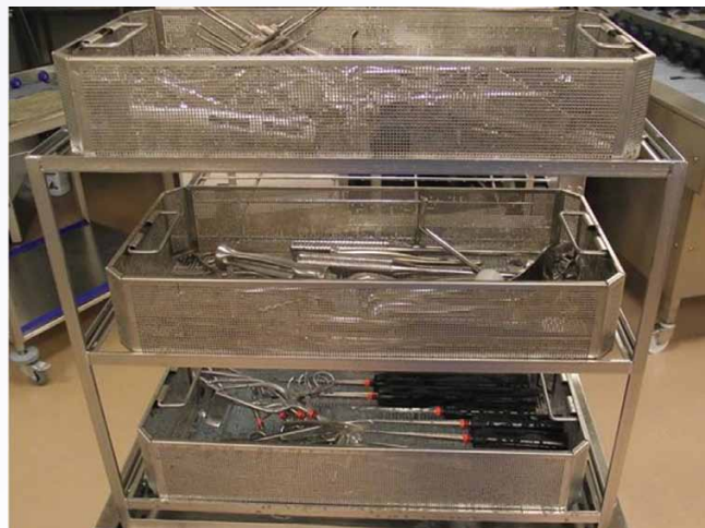
Figure 7. Correct loading of basket and instruments from rigid sterilization container in washer-disinfector
