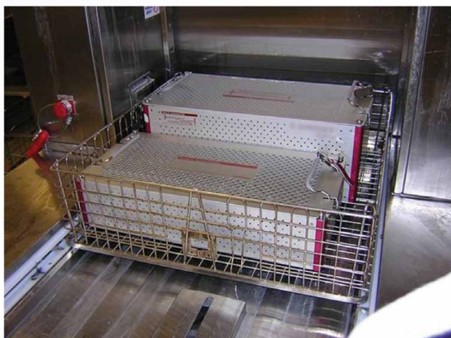
Figure 4. Loaner instrument containment devices improperly loaded into a washer-disinfector
