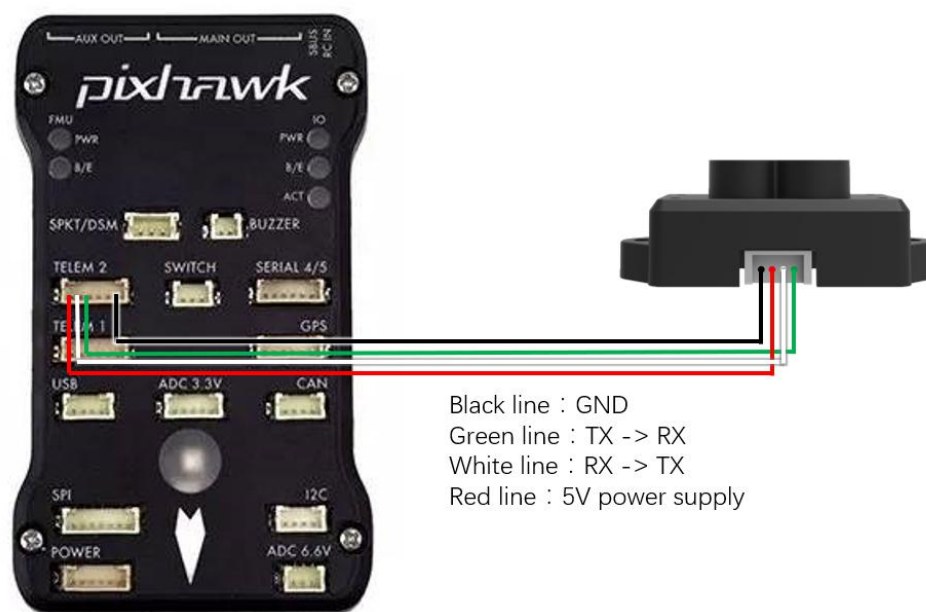
Figure 1: Schematic Diagram of Connecting TFmini with TELEM2 (Serial Port 2) of Pixhawk
