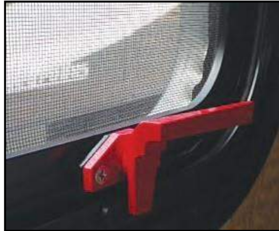
Figure 2-9: Emergency Exit Latch
