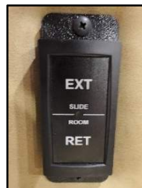
Figure 10-2: Front Slide-Out Switch
