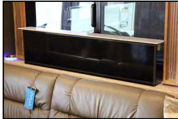
Figure 6-6: Television Lift (Lifting)
