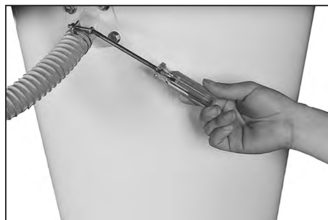
Figure 17. Cyclone vacuum tube and hose attachment.
