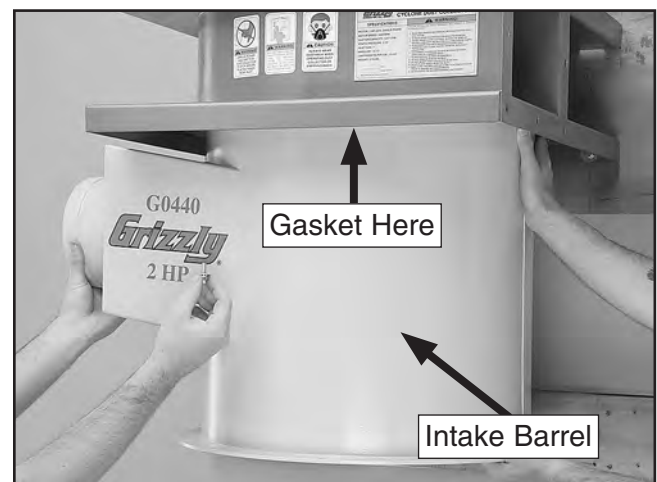
Figure 13. Example of securing blower on intake barrel.
