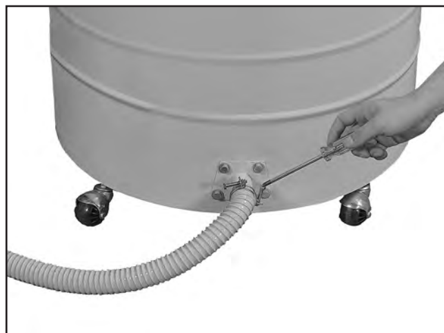
Figure 29. Connecting the vacuum hose.
