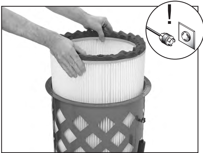
Figure 62. Removing the filter from the canister assembly.
