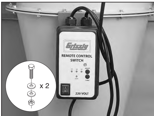
Figure 31. Magnetic switch mounted to funnel.
