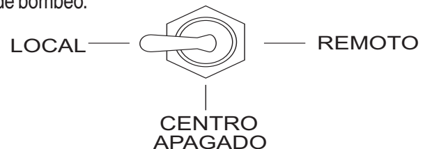
Figura 26. Interruptor de control de bombeo (LOCAL)
