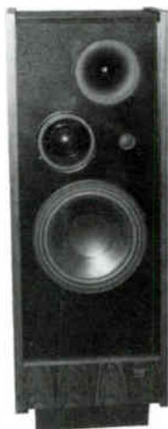
The AEC Monitor loudspeaker. The bright spot inside the tweeter is the glow of the plasma.
