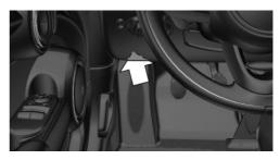
There is an OBD socket on the driver's side for checking the primary components in the vehicle's emissions.
