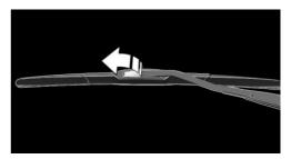
4. Pull the wiper blade down out of the holder on the wiper arm, arrow 1.
