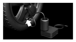
5. With the compressor switched off, insert the connector into the power socket in the vehicle interior.
