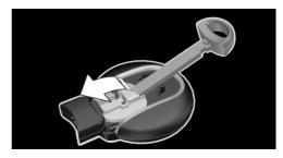
4. Push battery in arrow direction using a pointed object and lift it out.
