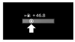
The bar display below the tachometer is filled in green and the mark appears at the zero point. The tachometer indicates idle speed.
