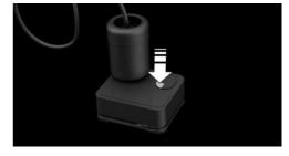
Let the compressor run for max. 10 minutes to fill the tire with sealant and achieve a tire inflation pressure of approx. 2.5 bar. While the tire is being filled with sealant, the tire inflation pressure may sporadically reach approx. 5 bar. Do not switch off the
