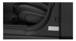
The vehicle identification number can be found on the nameplate, on the left-hand side of the vehicle.
