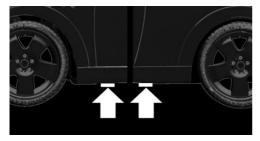
The jacking points for the vehicle jack are located at the marked positions.
