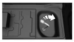
4. Unlock the locking hexagon of the emergency wheel well using the hexagon attached to retaining plate.
