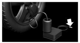
6. With the ignition switched on or the engine running, switch on the compressor.
