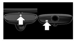
Photocells are used for control:
