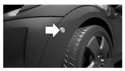
The ultrasound sensors for measuring parking spaces are located on the wheel housing.
