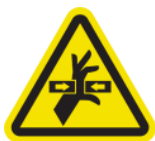
Hazardous moving part
