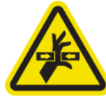
Hazardous moving part
